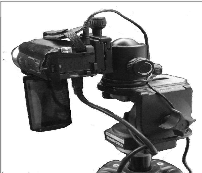
*Illustration 1: HD camera tilted 90° using a Ball-head*
