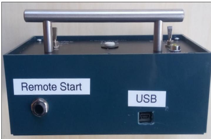
**USB** is used to connect the Control box to the computer using a standard USB cable.
